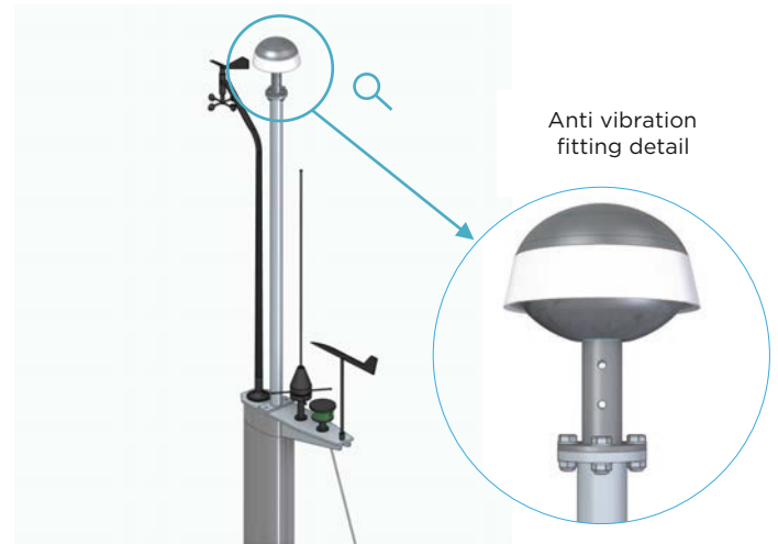
Figure 8. Standard mast installation.
